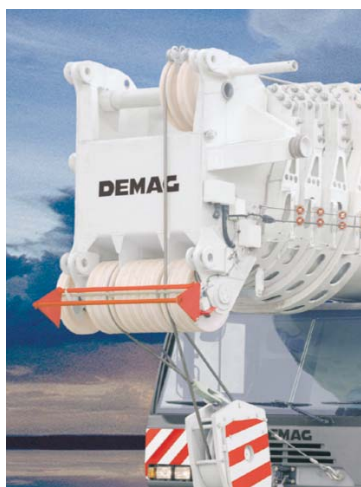
Boom head of an AC 500-1 mobile crane with sheaves made of cast nylon. (Photo courtesy of Demag Mobile Cranes GmbH.)
