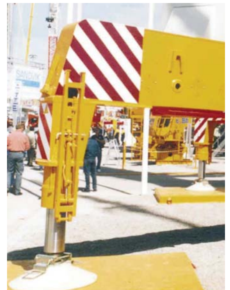
Outrigger float pad made of cast nylon 6/12. (Photo courtesy of Demag Mobile Cranes GmbH.)
