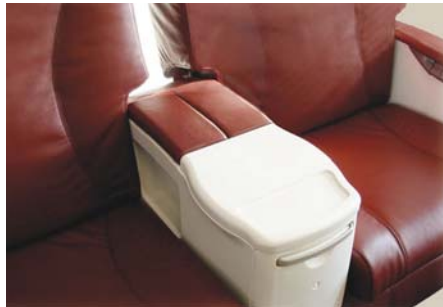
The plastic components of this aircraft seat were made using Boltaron 9815E, a proprietary, thin gauge film that meets stringent FAR 25.853 (a)(d) requirements for flammability, smoke density and heat release.
