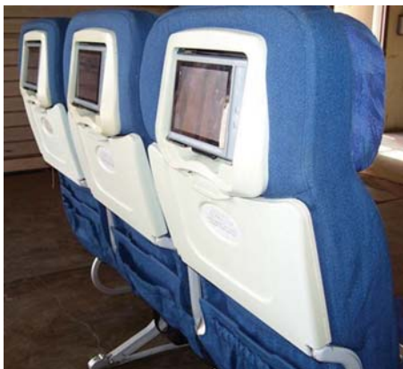
The plastic components of this aircraft seat were thermoformed with Boltaron 4330 sold through one of its international distribution partners. Boltaron 4330 meets FAR 25.853 (a) flammability requirements.
