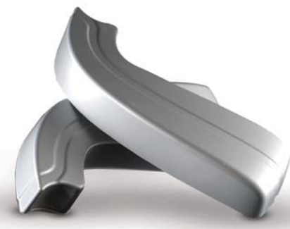
Aircraft armrest thermoformed using Boltaron 9815M, a proprietary, FAR 25.853 (a) and (d) rated, PVC/acrylic alloy that meets FAA requirements for flame, heat release and smoke generation.
