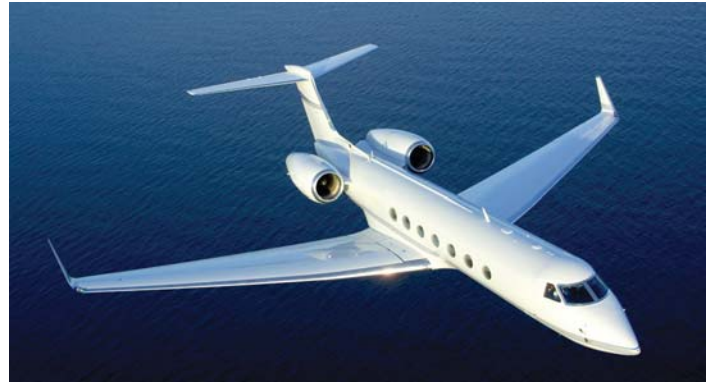
Gulfstream G650 business jet with its first-of-kind welded thermoplastic composite rudder and elevator tail section based on a Fortron® polyphenylene sulfide (PPS) matrix developed by Royal Ten Cate.
