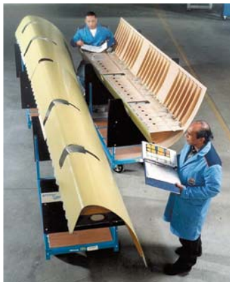
Fortron® based PPS composites are used in demanding aerospace applications like this Airbus A380 leading edge. It was selected for its low cost and excellent performance in this critical environment.
