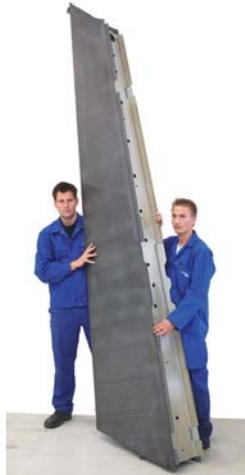
Gulfstream G650 business jet with its first-of-kind welded thermoplastic composite rudder and elevator tail section based on a Fortron® polyphenylene sulfide (PPS) matrix developed by Royal Ten Cate.
