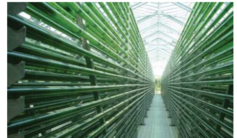
The use of tubular photobioreactors consisting of long horizontal tubes eliminates the problem of shadowing.
