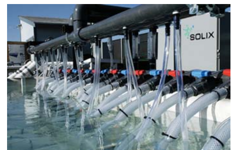
Example of an open system photobioreactor.
