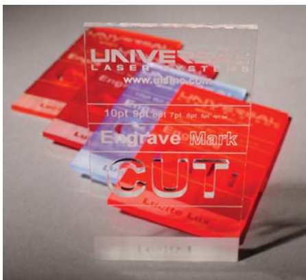
Figure 1. Raster engraving, vector engraving and cutting LuciteLux™ sheet in a single laser processing operation.
