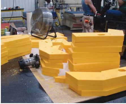
Every part was CNC milled, pre-drilled, coded and then hand routed to remove sharp edges.
