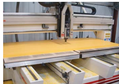
The custom made 2" thick HDPE sheets were CNC milled to create the 720 parts of the sculpture.
