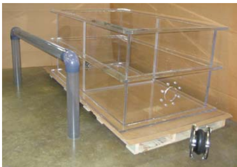
Clear rectangular acrylic tank which is joined to the piping with a conventional expansion joint.
