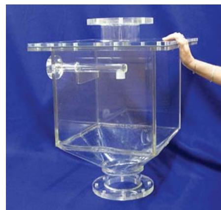
Figure 2. Rectangular acrylic vessel with a removable lid and a tapered bottom.
