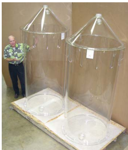
Figure 1. John Cox of PLASTICO displays an acrylic tank used in the revitalization of ion exchange resin used in deionized water applications.
