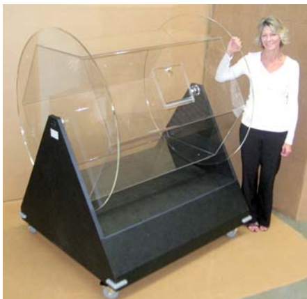
Figure 4. Karen Sadler of PLASTICO displays a tumbler fabricated with an ABS covered wooden base, line bent acrylic body and acrylic cylindrical end panels.
