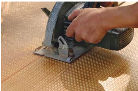
Unlike shelters that rely on concrete and steel, the wall sheathing of the Norplex-Micarta StormBlocker™ composite-based system is relatively thin and easy to cut.
