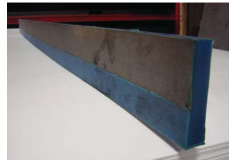
Wiper made of a 75-85A durometer urethane molded onto a 10-gauge steel bar that is plug welded onto the bottom of the scraper.
