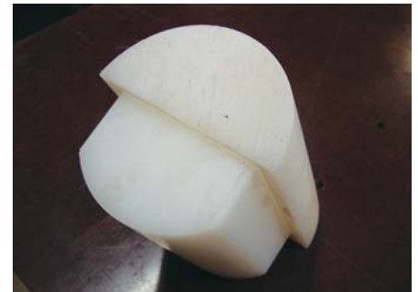
Guide machined with UHMW-PE and bolted into the end of each arm of the scraper.
