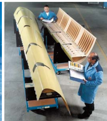
Airbus A340-500 and -600 planes use Ticona's Fortron® PPS thermoplastic composites in wing and other structural parts, replacing aluminum to decrease weight, improve impact resistance and ease fabrication.
