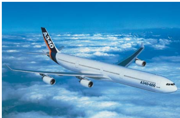
Airbus A340-500 and -600 planes use Ticona's Fortron® PPS thermoplastic composites in wing and other structural parts, replacing aluminum to decrease weight, improve impact resistance and ease fabrication.
