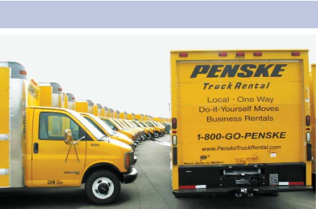
A roll-up door built with polyethylene custom run in the Penske yellow color.
