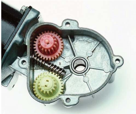
The motor power in this windshield wiper drive is transmitted via two worms to two cluster gears made from Hostaform® acetal copolymer, grade C 9021. The cluster gears have helical gears mated to the worms and spur gears driving a single output gear (not shown).
