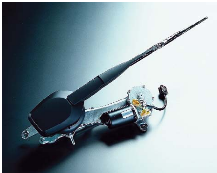
Mercedes Benz single-arm windshield wiper system. Drive and wiper arm covers are injection molded from Ticona's impact-modified, weather-resistant, UV-stable Hostaform® acetal copolymer.
