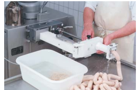
Components made from various plastics in a sausage machine. Photo: Vernag GmbH, Germany.
