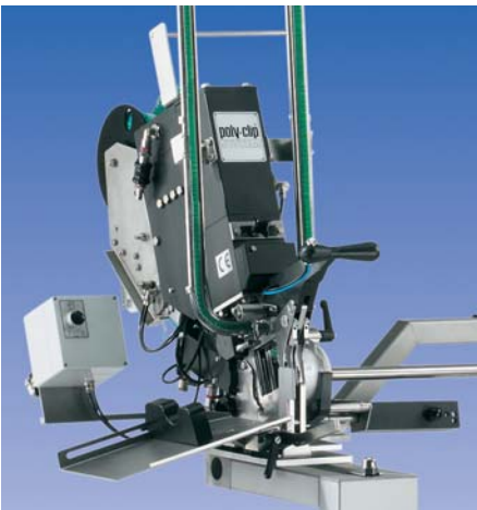
Components made of ZL 900 (acetal) in a sausage processing machine. Photo: Poly-Clip GmbH, Germany.
